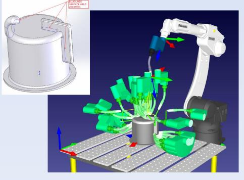
With RoboDK it is possible to use robots as a 3D printer or like a CNC. It is very easy to generate robot programs for applications such as milling, welding, painting, deburring, ... You can easily simulate and convert CNC programs into robot programs. RoboDK will automatically optimize the path planning, avoiding singularities, axis limits and collisions.
