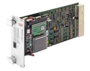
The SPiiPlusNT (NT - Network Controller) is designed for incorporation in the MC4U. Once plugged into an MC4U, the MC4U becomes also an EtherCAT master designated MC4Unt. It manages the EtherCAT network with up to 64 axes of motion and countless number of I/Os and sensor modules. The SPiiPlusNT also includes Servo Processors for controlling local drives that reside within the same MC4Unt enclosure.
