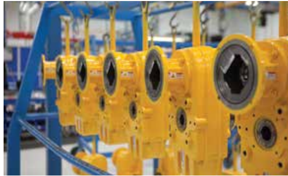
Assembly stages of “F” Series gearheads: Paint curing oven allows for one day assembly and higher paint durability (left); units awaiting final inspection prior to shipment (right).
