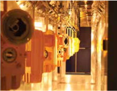
Assembly stages of “F” Series gearheads: Paint curing oven allows for one day assembly and higher paint durability (left); units awaiting final inspection prior to shipment (right).
