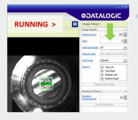
NO MONITORING DOWNTIME The monitoring tool offers the possibility to adjust parameters in-line, without disconnecting the reader from the host communication or accessing the setup area.
