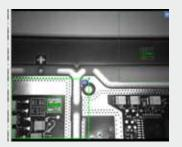
MULTIPLE CODE OPTI-MIZATIONS Multiple decoding regions improve reading speed with multiple code applications or independent codes with different features.
