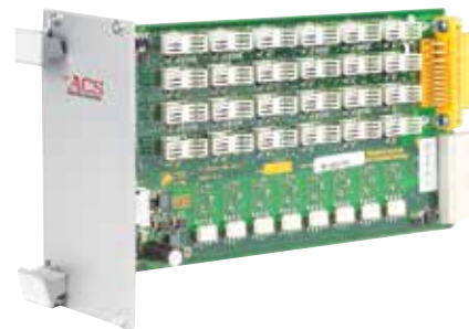
DDM3U-4-60V Up to 4 Universal Drives per Card 60V, 5A peak, 0.3kW
