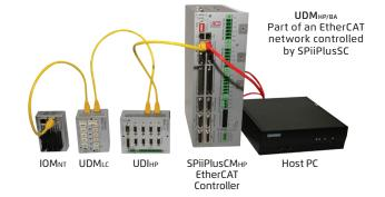
The UDM<sub>HP/BA</sub> addresses high accuracy demanding applications, while the UDM<sub>HP/BA</sub> econo version addresses more price sensitive applications. The UDM<sub>HP/BA</sub> are complemented by the SPiiPlusNT suite of software tools that minimizes network configuration and drive set up efforts and time to market. The built-in drives are offered with three current levels: 5/10A, 10/20A and 15/30A ((cont./peak).
