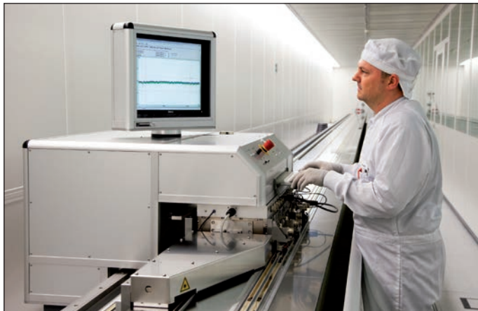
30 m long measuring machine for scale tapes
