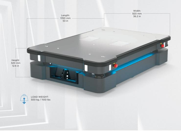
**MiR**500 is designed to automate the transportation of pallets and heavy loads across industries. With a payload of 500 kg and a footprint of 1350x920 mm, MiR500 is the largest, most powerful robust collaborative, autonomous mobile robot from MiR.
