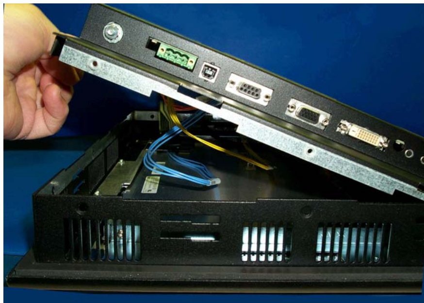
Figure 4-1: Removing the 15" Monitor Back Cover
