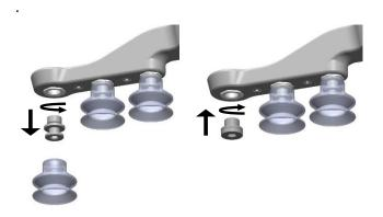
The thread size is the commonly used G1/8"; allowing for standard fittings, blinders and extenders to be fitted directly to the VG grippers.
