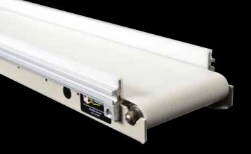
Side rails can be used to contain and guide product on the conveyor. They are available in 1/3", 1" (shown) and 2". You may also order them with seals to keep product or contaminants from slipping under the belt or with a wear strip to protect the sides and product from scuffs and marks.
