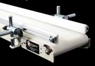
Adjustable side rails offer the ultimate in flexibility. These guides may be adjusted vertically for varying product heights or horizontally to create full width or indented guides. These guides are available with optional thumb screws (shown) for tool-less adjustments.
