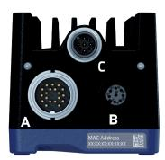
A - M16 Male 19 poles (I/O & Power) B - M12 Female 8 poles A-Coded (Gigabit Ethernet) C - M12 Male 8 poles A-Coded (Not Used)
